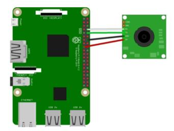
Camera 5V (black wire) to PI 3V or 5V Camera GND (black wire) to Pi Ground Camera RX (white wire) to Pi TX Camera TX (green wire) to Pi RX
