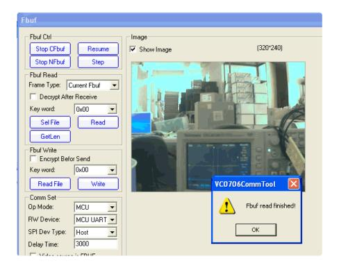
Thats it! You can now easily test reading camera images. To take another photo. Press **Resume** up at the top to have the video start up again. Then click **Stop CFbuf** when you want to snap another photo. Finally you can select the **Compression Ratio** which will improve or degrade the image quality but also change the image transfer time. There's no way to change the image size from this program (easily) but we can do it using the Arduino sketch so just try it out here to start.
