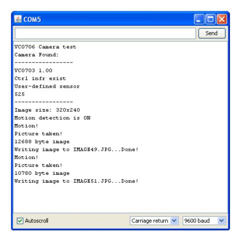
You can turn motion detection on or off by calling setMotionDetect()
